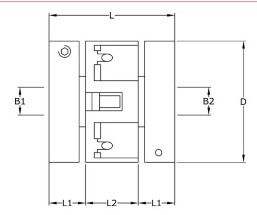
$\begin{array}{lll} B1 & = 5 \\ B2 & = 5 \\ D & = 27 \\ L & = 25.4 \\ L1 & = 9.3 \\ L2 & = 6.9 \\ Screw = M3 \end{array}$
